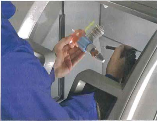
The integrated air pen lets you remove excess powder from the model under negative pressure — that excess is then recycled and reused automatically.
